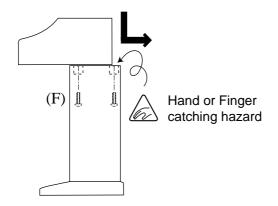
3. Place the piano on the front half of the stand so that the metal fitting holes are seen when viewed from the top. Slide the piano backward while holding it with one hand so that it does not incline and fall from the stand. The hooks on the piano are then engaged with the metal fittings on the Side Panels. Pay attention so that your hand or fingers are not caught between the stand and piano. Fasten the piano and the stand with four bolts(F).
